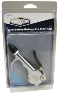
The rubber tip will not scratch or mar delicate surfaces. The conical rubber tip can also be used to create a seal between the blow gun and fluid lines (or any other opening). The base of the tip is nickel-plated brass for additional corrosion resistance. *Must be used on air lines having a maximum regulated pressure of 30 PSI in order to comply with OSHA Standard 1910.242 (B). Safety glasses or shield must be worn when using any blow gun.*
